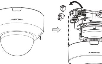
② Remove the enclosure from the camera. and power cord plug attached to the
