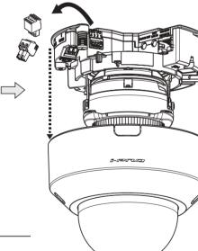
Remove the external I/O terminal plug camera
