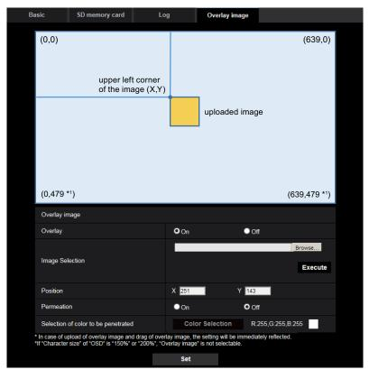
\*1 In case that [4:3] is set for [Image capture mode] When [16:9] is set for [Image capture mode], [Y] will be "359"
