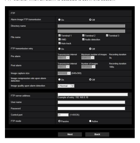
Refer to page 203 for information about how to set the above screen. For information about "Image compression rate upon alarm detection" and "Image quality upon alarm detection", refer to "2.7.4.2 Configure settings relating to image quality on alarm action".
