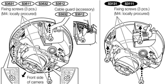
\* Tighten the 2 fixing screws on the lens side by using the slotted holes on the front side of the camera.
