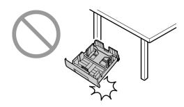
Hold the paper input tray with both hands when removing or installing. The paper input tray weighs approximately 2 kg when fully loaded with recording paper.
