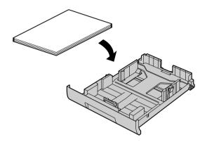
3 Insert the paper input tray into the unit, lifting the front part of the tray. Then push it completely into the unit.
