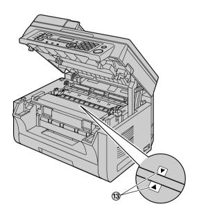
8 Close the top cover by holding the indentations on both sides of the unit, until locked.
