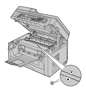
6 Close the top cover by holding the indentations on both sides of the unit, until locked.
