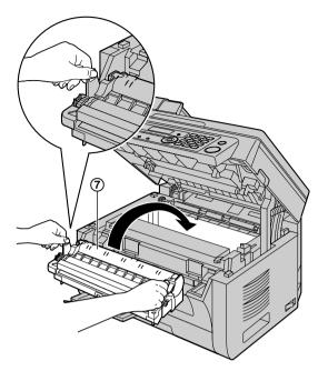
• Make sure that the arrows (®) match, to install the drum and toner cartridge correctly.
