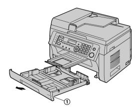
Before loading a stack of paper, fan the paper to prevent paper jams.
