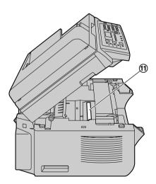
7 Install the drum and toner cartridge (⑫) by holding the tabs.
