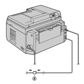
A telephone handset cannot be connected directly to this unit. To talk to the other party, please connect an extension telephone (KX-MB2025/KX-MB2030 only).
