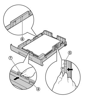
Insert the paper input tray into the unit, lifting the front part of the tray. Then push it completely into the unit.
