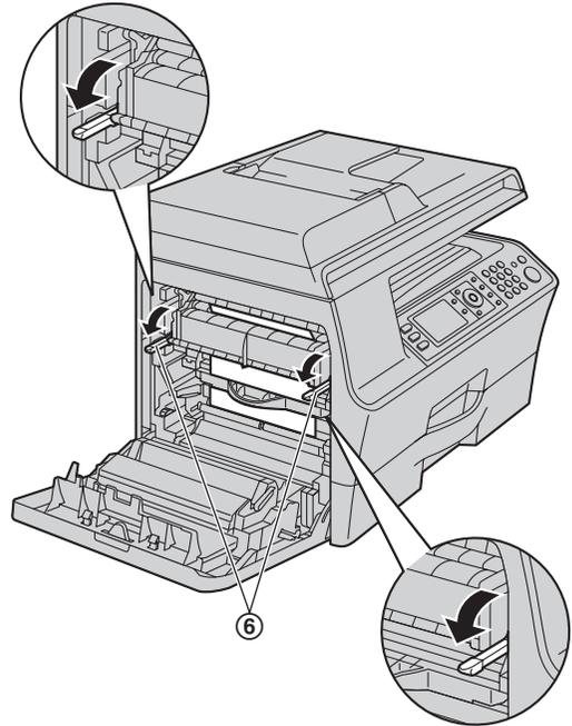
2. **When the recording paper has jammed inside the fuser unit:**
