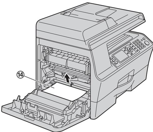
**When the recording paper has jammed near the automatic duplex unit:**
