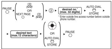
Similar to the above procedure, when storing other types of buttons (CO buttons, feature buttons, etc.), the displayed text for the Self Labeling LCD Display can be assigned.
