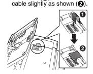
Attach the KX-NT303 to your unit with the screws (included with KX-NT303).
