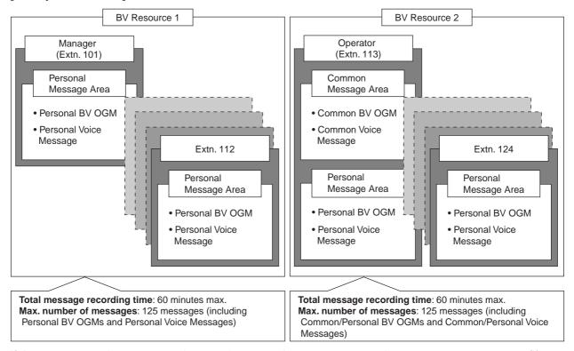
If there are new voice messages in a user's personal message area or the common message area (if accessible), the user will hear a special dial tone (dial tone 4) when going off-hook. In addition, if that user's telephone has a MESSAGE button or Message/Ringer Lamp, the corresponding button or lamp will light
