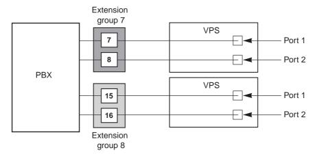
This example uses a Panasonic KX-TVM50/KX-TVP50 VPS, which can be connected with 4-conductor wire to 4 extension jacks of the PBX.
