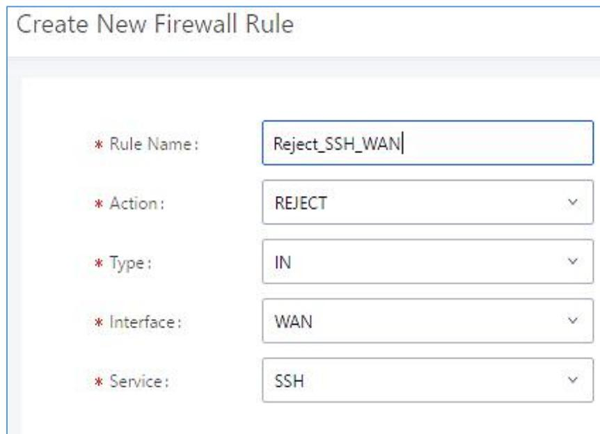
**Figure 28: Create New Firewall Rule**
