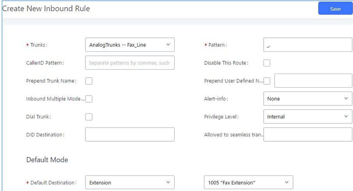
**Figure 204: Configure Inbound Rule for Fax**
