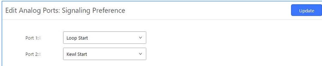
**Figure 251: FXS Ports Signaling Preference**
