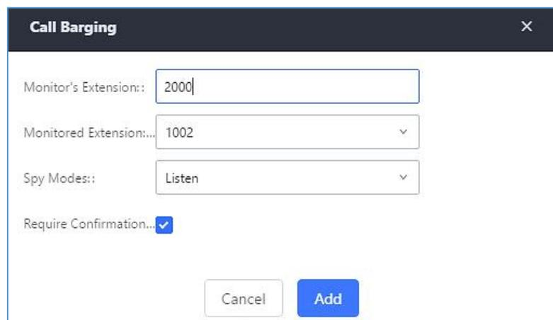
**Figure 229: Configure to Monitor an Active Call**
