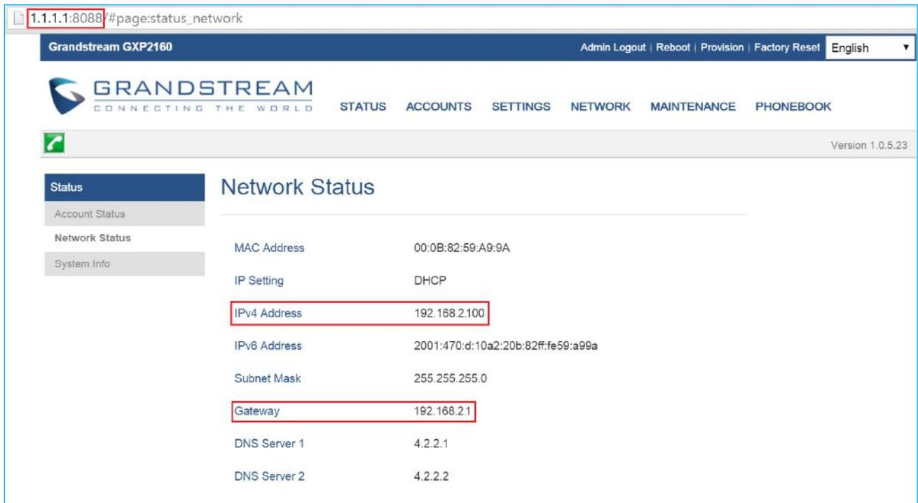
**Figure 23: GXP2160 Web Access using UCM6202 Port Forwarding**
