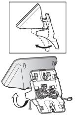
5 Mount the unit on a wall then slide down to secure in place.AC adaptor cord
