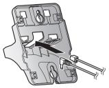
2 Tuck the telephone line cord inside the wall mounting adaptor (1). Connect the AC adaptor cord and telephone line cord (2).
