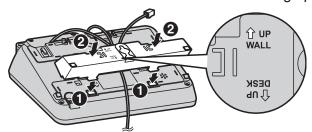
4 Mount the unit on a wall then slide down to secure in place.
