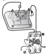
3 Insert the hooks on the wall mounting adaptor into holes ((a)) and ((b)) on the base unit.
